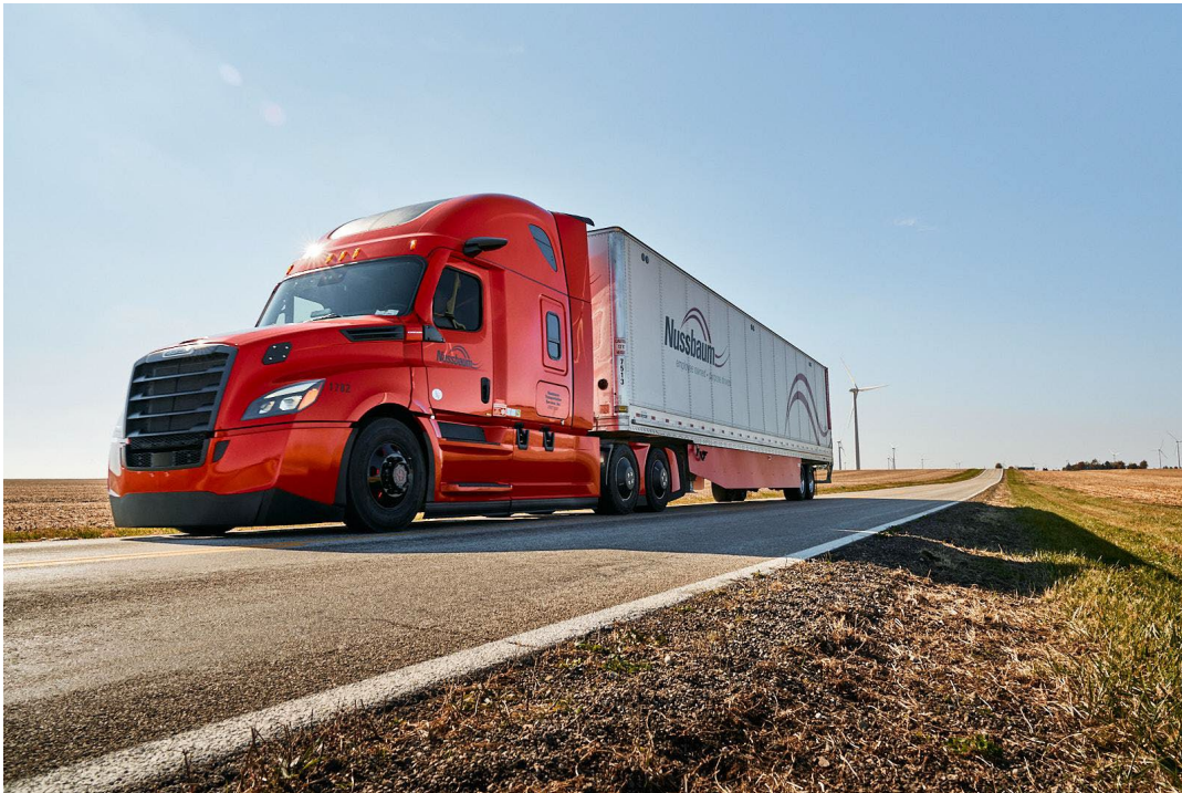
Figure 16: Top fleets like Nussbaum adopt a variety of technologies to improve freight efficiency. Nussbaum is now using cameras instead of mirrors on some of its trucks for an additional 1.5% fuel economy gain. (Photo: Nussbaum)
