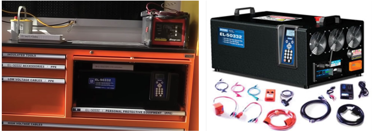
Figure 71. Left, battery cell levelling tool in cabinet (Weber State). Right, example battery discharge/load levelling tool (GM).
