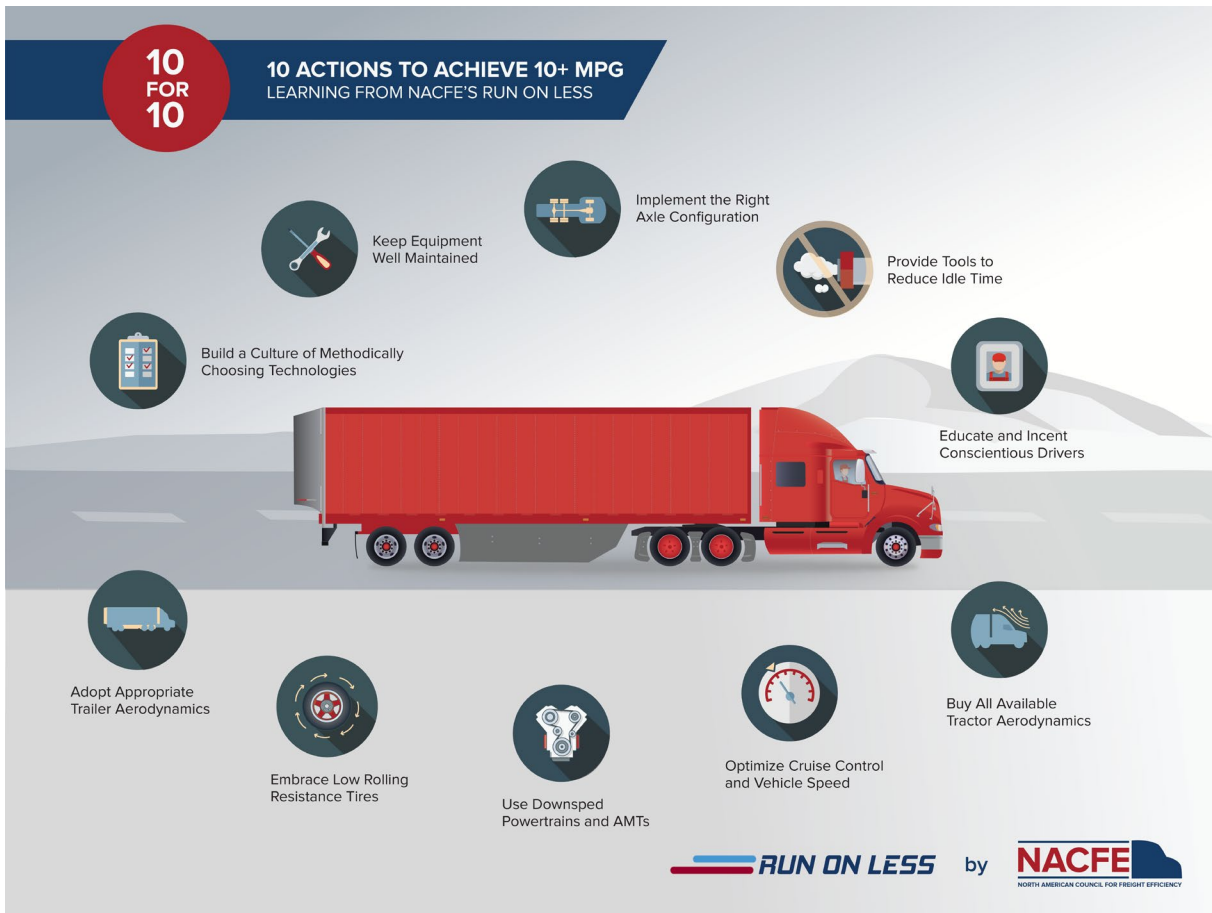
Figure 37. Factors for efficiency improvement of diesels, many applicable to BEVs (Click here for a larger version of this graphic.)
