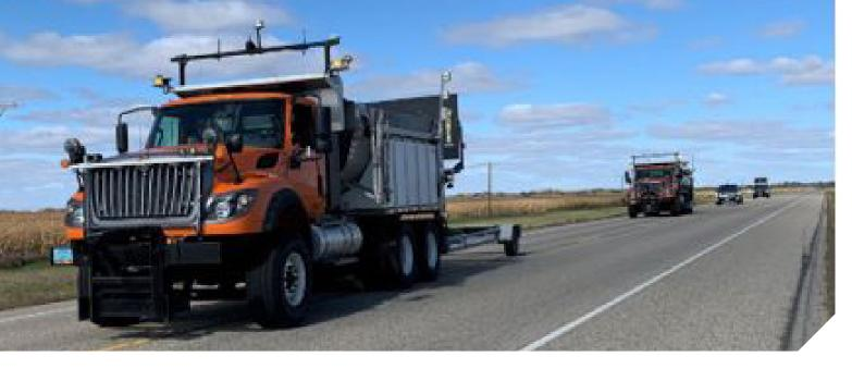
Kratos Defense has developed a platoon crash-barrier truck for use in highway construction applications and is now working on freight-hauling systems as well.
