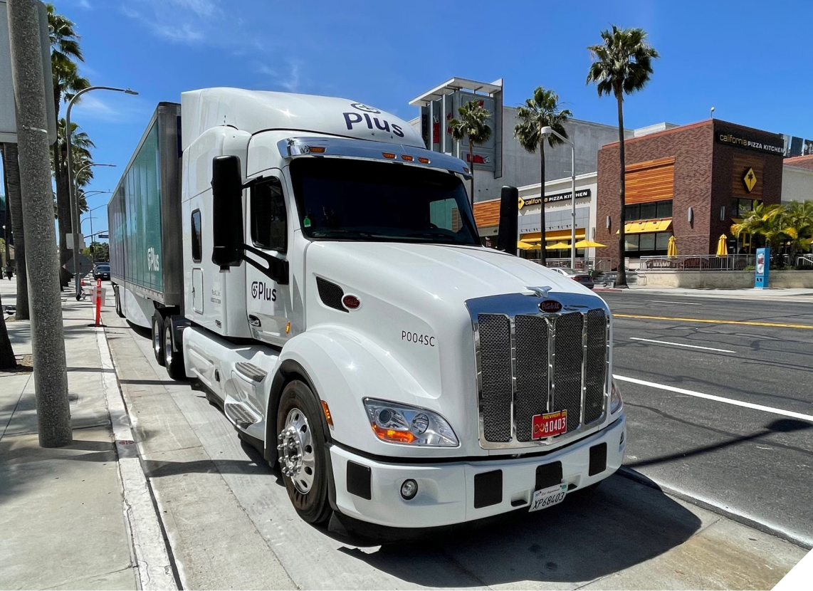
A Peterbilt Model 579 tractor retrofitted with Plus AI's "PlusDrive" autonomous control system, awaits another freeway run outside the Long Beach Convention Center during ACT Expo 2022.
