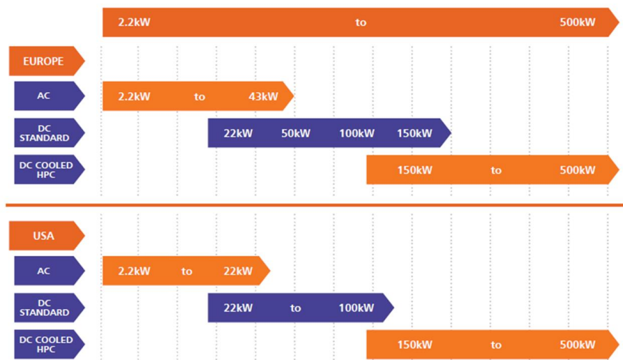
Figure 16. Liquid Cooled Cables Enable Higher Level Charging (ITT Cannon)[22]
