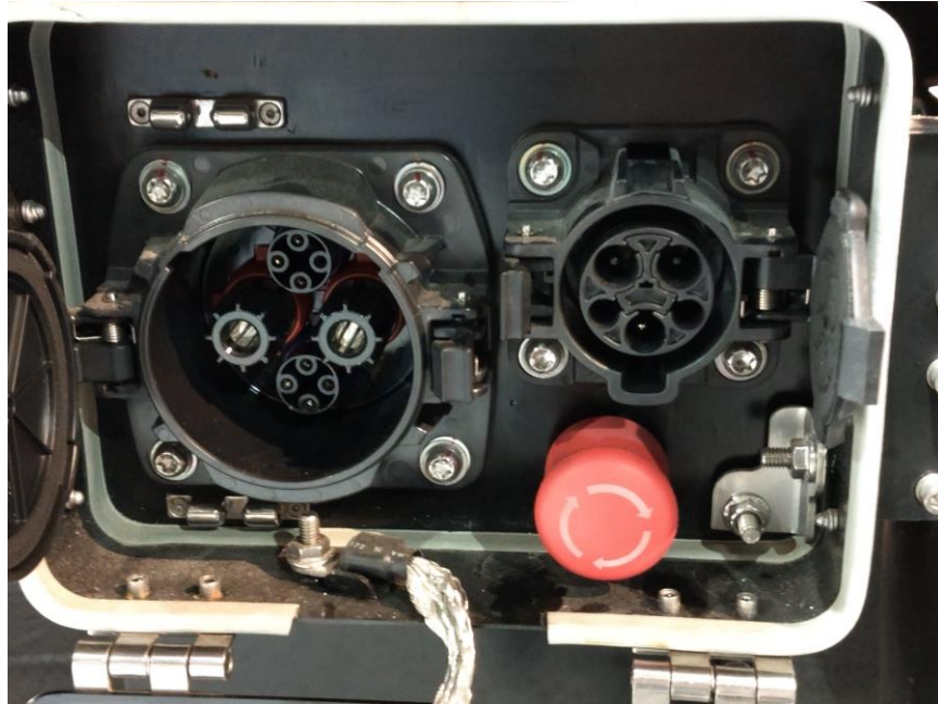
Figure 13. Mitsubishi Fuso eCanter J1772 and CHAdeMO Charging Connections (Mihelic) [[18]
