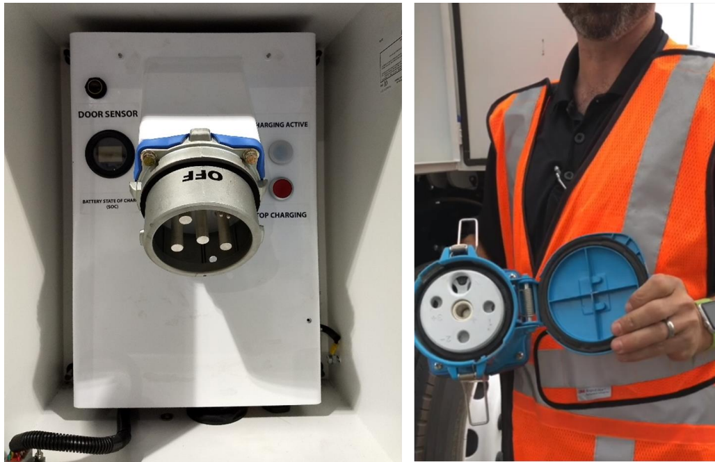
Figure 14. TransPower EV Yard Tractor 208V Connector (Mihelic, TransPower) [18][19]
