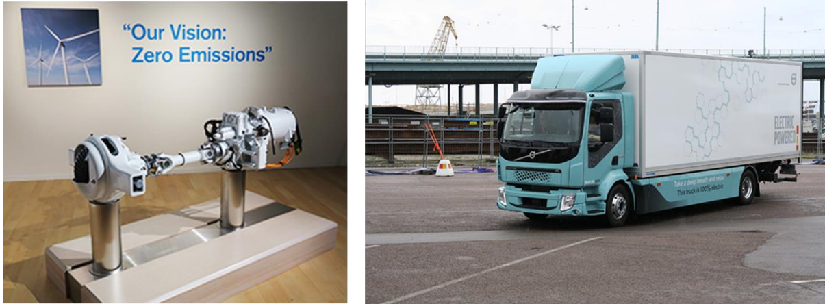
Figure 110. Volvo Electric FL with Electric Driveline (Seth Clevenger) [256]
