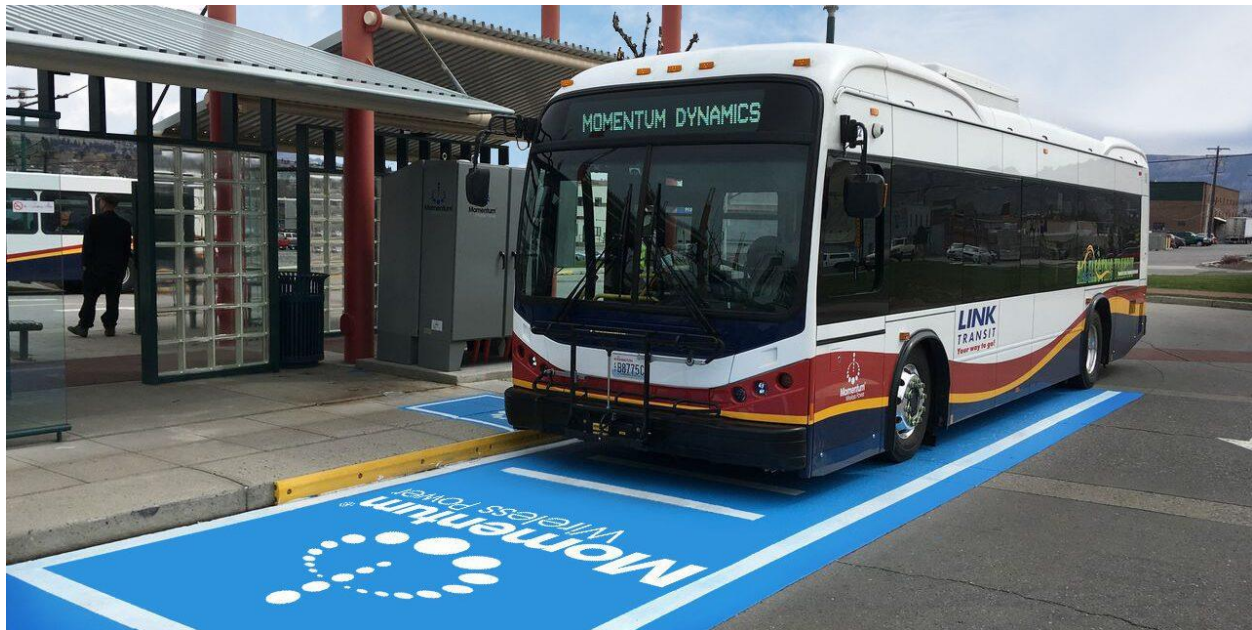
Figure 19. Example 200kW Wireless Charging (Momentum Dynamics)[29]
