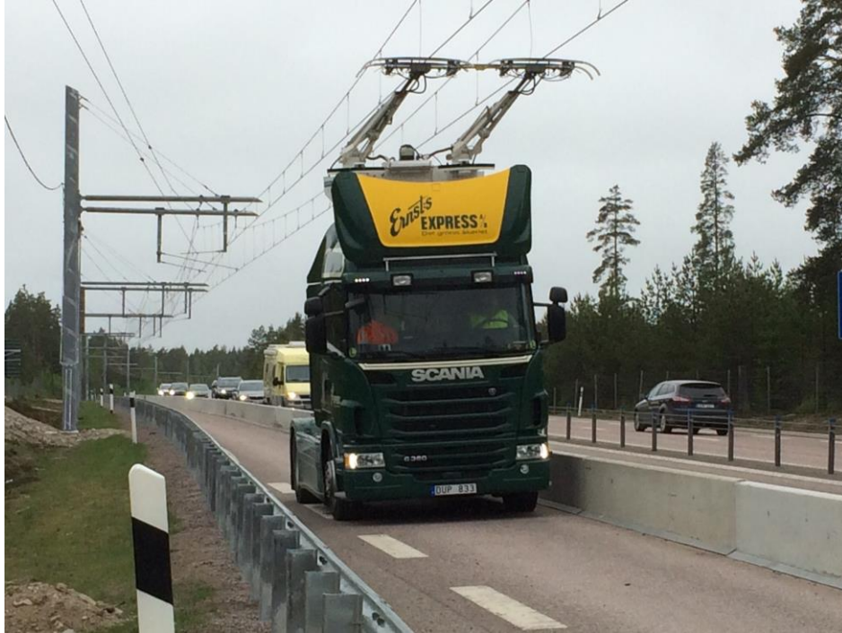
Figure 20. Overhead Conductive Charging (Trafikverket) [37]
