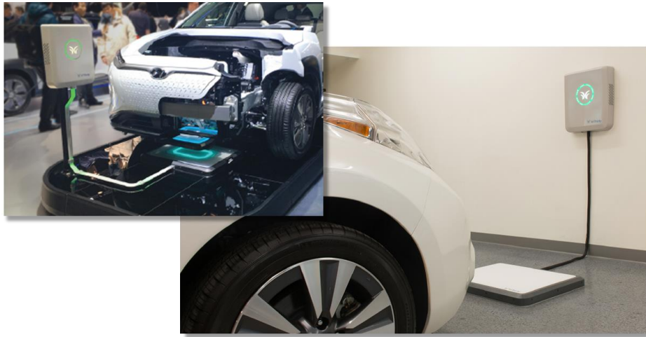
Figure 18. Example Magnetic Resonance Wireless Charging System (Wi Tricity) [26]
