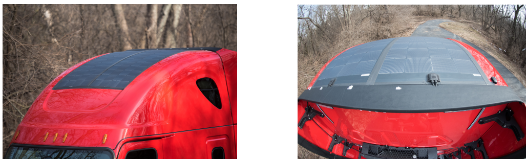
Figure 15: Solar panels mounted to the tractor fairing (Source: Bergstrom)
