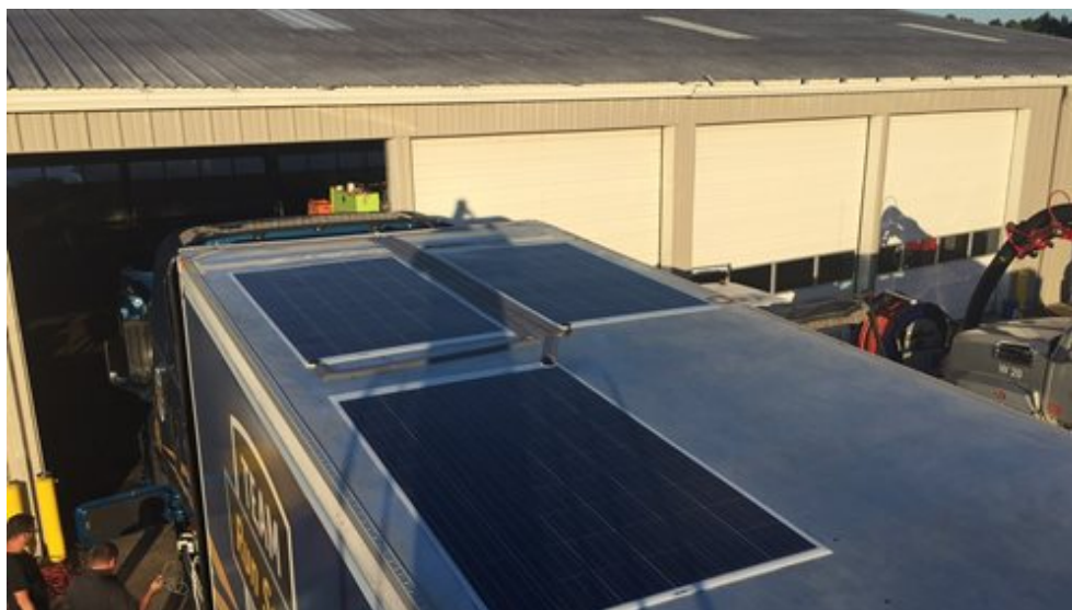
Figure 18: Solar Panels Mounted to Trailer Roof (Source: Team Run Smart 11 )
