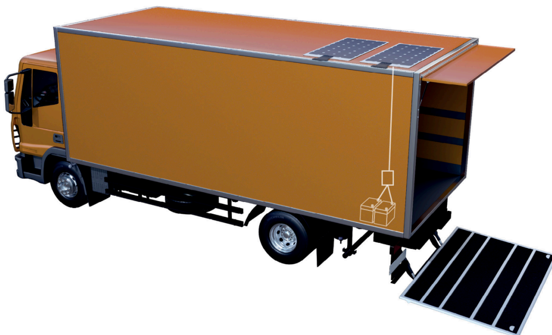
Figure 21: Solar panels mounted to the trailer to power a liftgate system (Source: Go Power! 14 )
