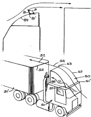
Figure 36 Roof Fairing Patent Image (Trailmobile)
