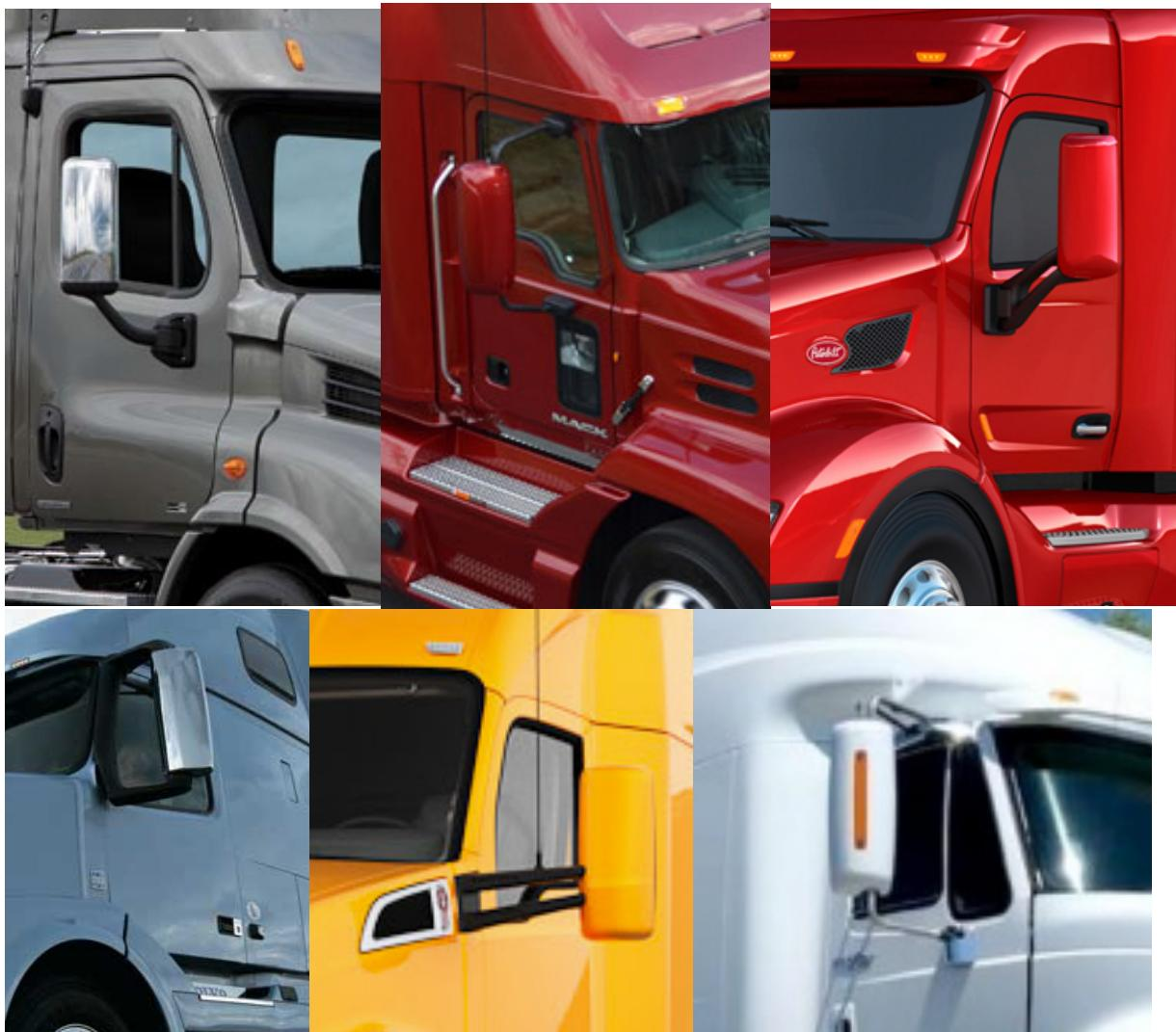
Figure 13 Examples of Aerodynamic Cab Mirrors and Mounting Arms
