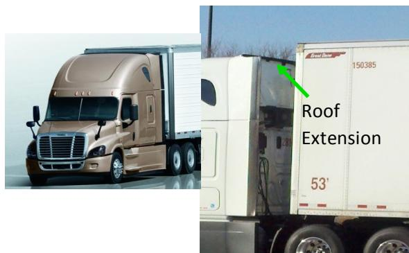
Figure 25 Freightliner Cascadia Roof Extension (Freightliner)
