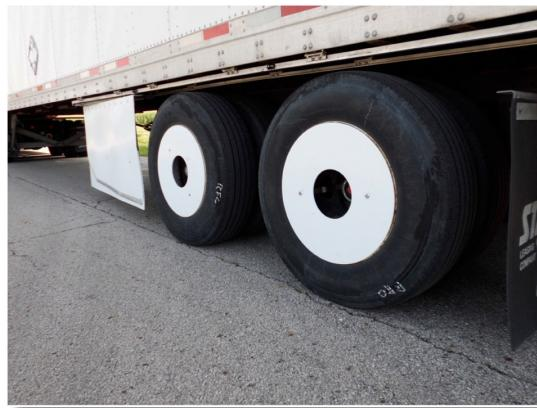
Figure 45 Solus Wheel Cavity Cover
