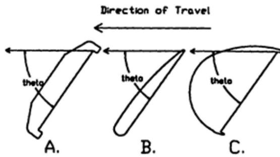
**Figure 4. Horizontal Cross-sections of Mirrors Investigated**
