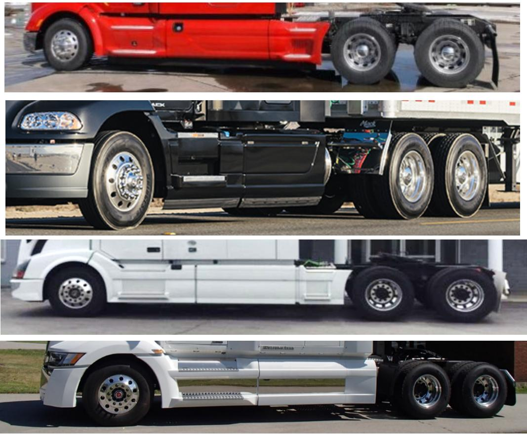
Figure 32 Sleeper Chassis Fairings – Peterbilt 579 full length with skirt, Mack Pinnacle with sleeper length skirt, Volvo VNL780 full length with steps, Western Star Sleeper length with extension.
