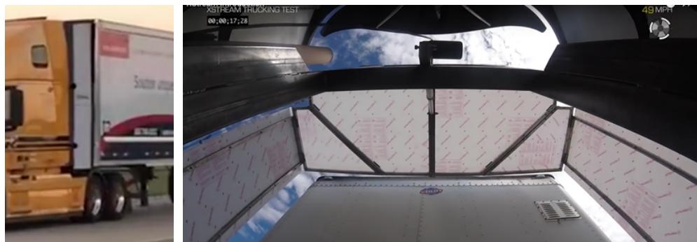
Figure 58 Deployable Gap Filler (XStreamTrucking)
