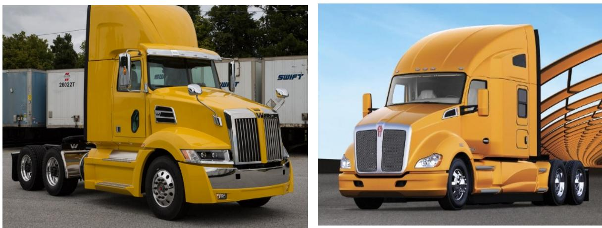
Figure 6 Day Cabs (left) and High Roof Sleepers (right) (Western Star & Kenworth)
