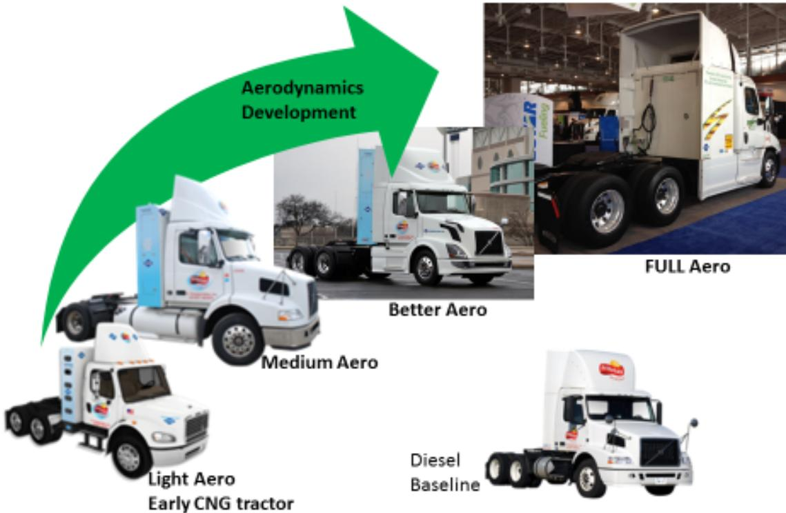
FIGURE 60: CNG Tractor Aero Evolution
