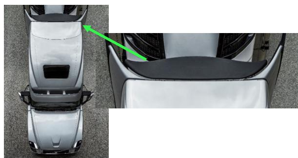
Figure 28 Volvo VNL680 Roof Extension (Volvo)
