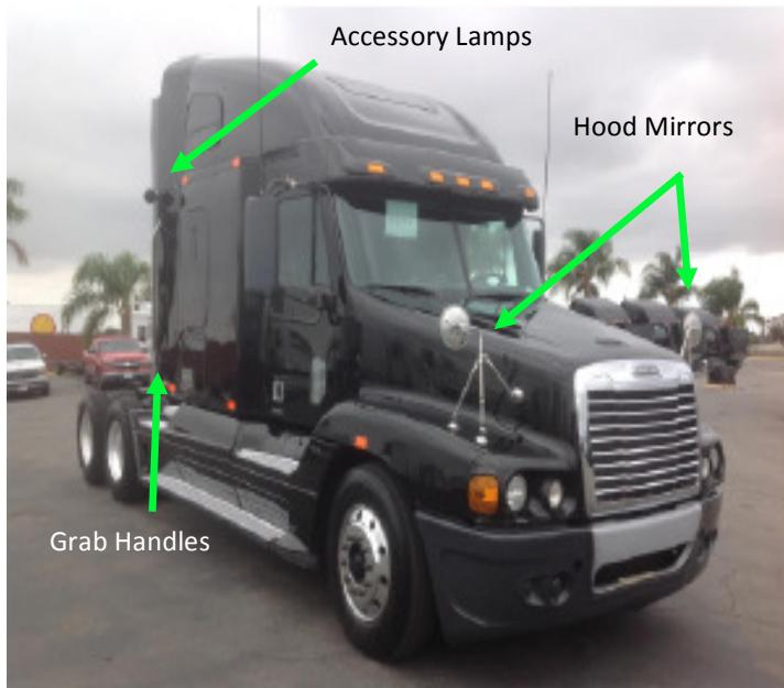
Figure 56 Options May Alter Aerodynamic Drag versus OEM Optimized Configuration
