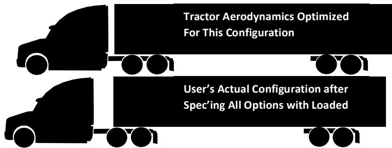
Figure 19 Frame Options Drive Tractor/Trailer Gap
