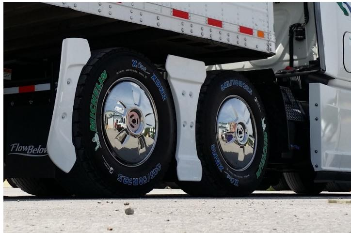
Figure 11 FlowBelow Drive Wheel Aero Kit and Wheel Covers
