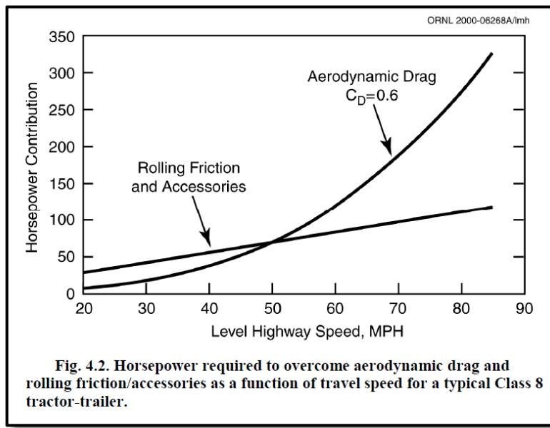
Figure 10 Horsepower vs. Speed (DOE circa 1998)
