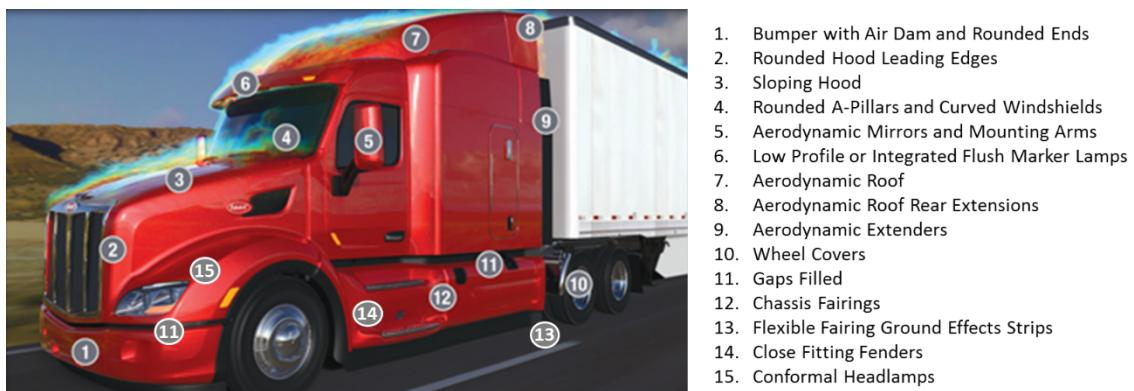
Figure 8 Elements of a Modern Aerodynamic Tractor (Peterbilt)
