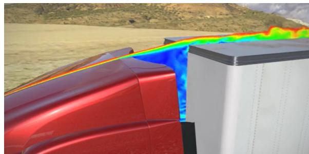
Figure 24 Analysis shows Roof Extension Helps Air to Jump Gap (Peterbilt) Navistar
