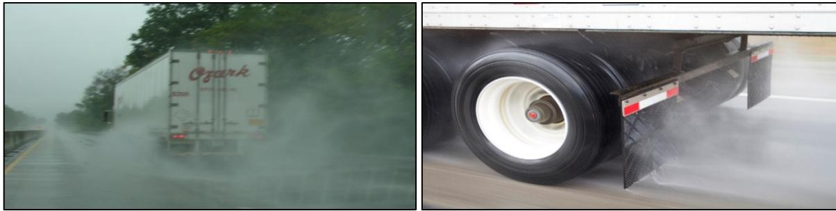
Figure 50 Mudflap Aerodynamic Effectiveness Can Be Seen in Wet Weather (photos courtesy of Cindy Kerr and Amy Hancock)
