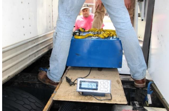
Weighing the test tank (no floor on this run)
