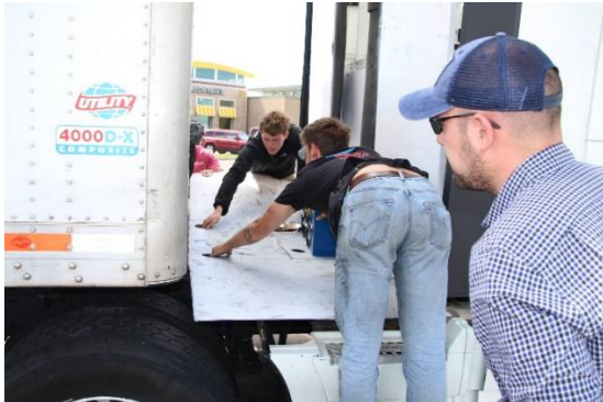
Installing the GapGorilla floor between runs
